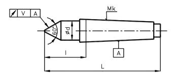
The centres serve to clamp workpieces on machine tools or check instruments. The centres of Nk=0-5 sizes are all hardened to HRC 58-62 hardness. On centres of Mk=6 size the tip is hardened along the length 80 mm while the remaining part is heat treated. The centres are made of tool steel. MORSE taper shank, ČSN 220420 (DIN 228, ISO 296) without clamping thread.
